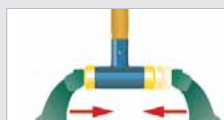
Simple replacement of outworn hammer faces: 1. Secure the hammer in the vice, lift away the old hammer face. 2. Press in the new hammer face in the vice.
