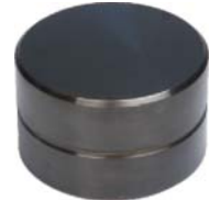
hardness test block (standard)
