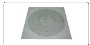
overlay chart (protractor with 1° graduation, radius with 1mm increment)
